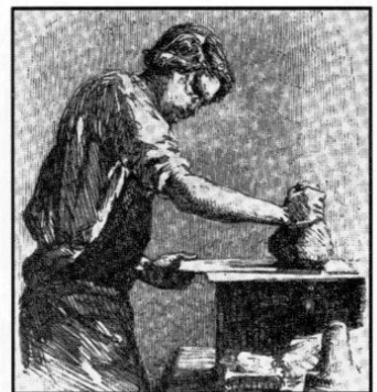
Figure 4. Inking a plate on a charcoal brazier, 1853. Courtesy of the Essay-Proof Society.
