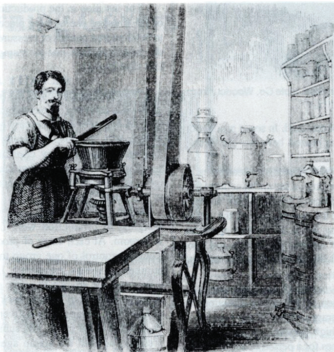
Figure 10. Ink mill for grinding pigments. Belt provides power from a stationary steam engine in another room. Harper's Monthly , 1862.
